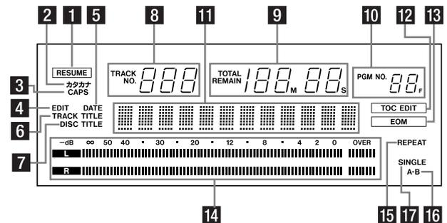
The different indicators and parts of the display are shown here. We refer to the parts of the display which light and show preset messages as "preset indicators" or simply "indicators".
